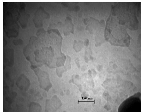
Figure 1. SEM image of KF/CP nanoparticles.
