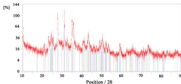
Figure 2. XRD spectra of KF/CP nanoparticles.
