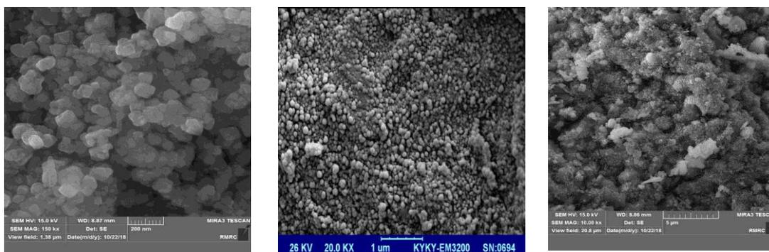
**Figure 1.** **1a.** SEM image of ZnO-NPs; **1b.** Fe<sub>3</sub>O<sub>4</sub>-MCNPs **1c.** Fe<sub>3</sub>O<sub>4</sub>/ZnO MCNPs.
