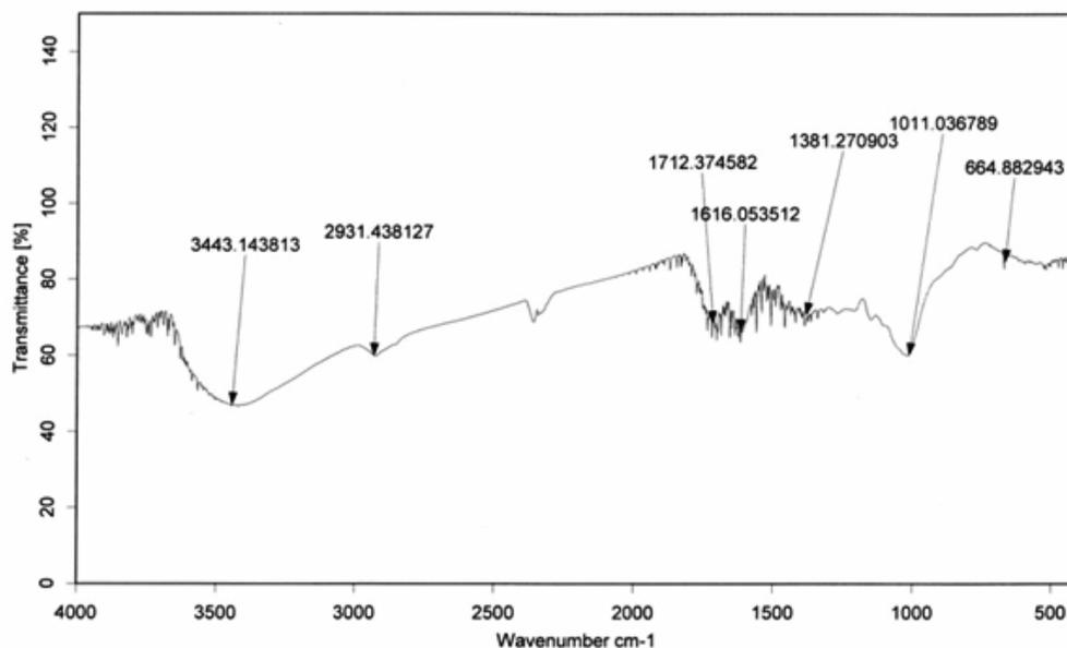
**Figure 3:** FT IR spectrum of  $\text{SbCl}_5/\text{nano-sawdust}$ .
