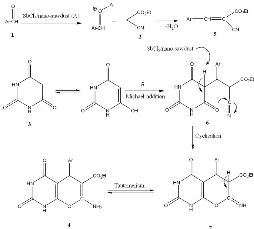
**Scheme 2:** Plausible mechanism for the formation of pyrano [2,3-d] pyrimidine derivatives.
