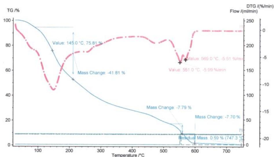
**Figure 2:** The TGA/DTG curves of SbCl<sub>5</sub>/nano-sawdust.
