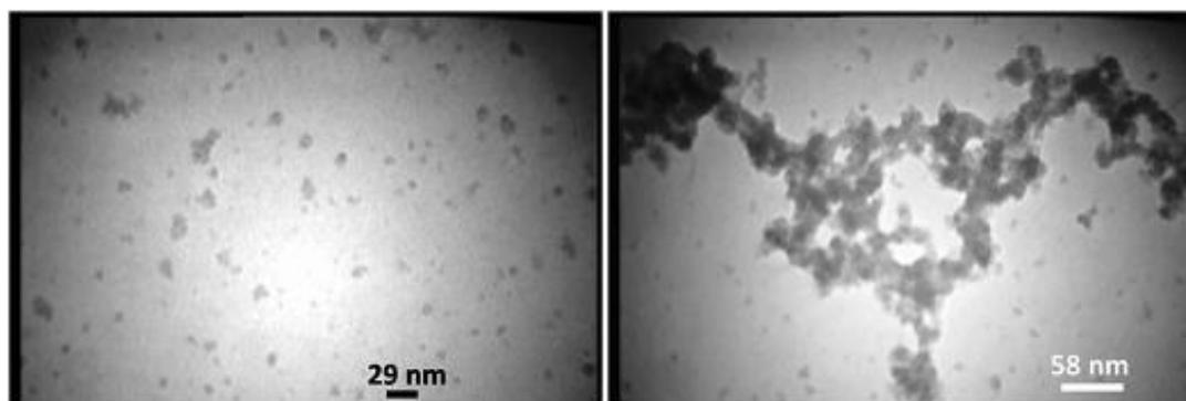
**Figure 1:** TEM micrograph of SbCl<sub>5</sub>/nano-sawdust.
