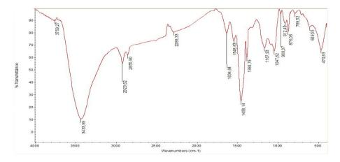
Figure 1: FT IR spectrum of Cu-PAA-PPy
