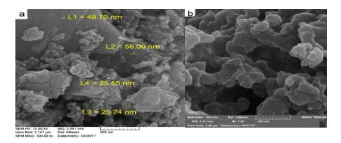
Figure 3. FESEM images of a) Cu b) Cu-PAA-PPynano composite
