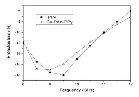
Figure 4: Microwave absorbing The results for PPy, Cu-PAA-PPy
