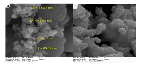
Figure 3: FESEM images of a) CI NPs and b) CI-PAA-PPynano composite
