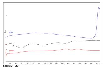
Figure 2: Comparing thermal behavior (DSC analysis) of PCSA1, PNSA1 and PTNSA1.
