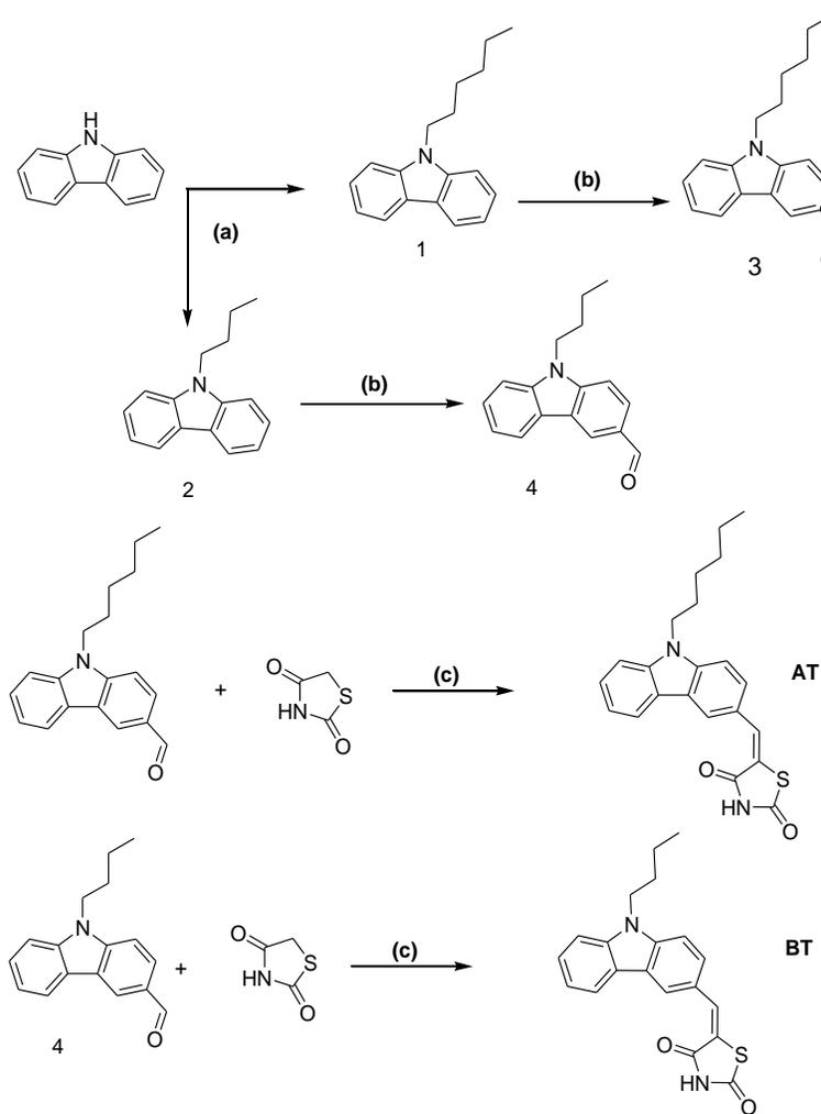
**Scheme 2:** Synthetic routes of AT and BT (a) 1-Bromoalkyl, NaOH, DMSO, 110 °C, overnight (b) POCl<sub>3</sub>, DMF, 95 °C, overnight (c) Acetic acid, Ammonium acetate, 90 °C, 10 h.
