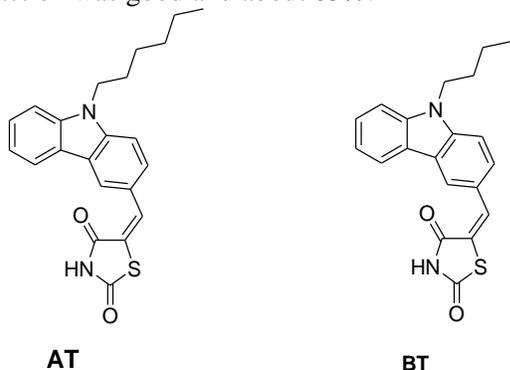
**Scheme 1:** Chemical structure of designed dyes AT and BT.
