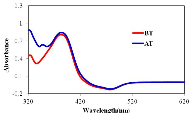
**Figure 1:** Absorption spectra of dyes AT and BT in THF.
