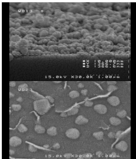
**Figure 4:** SEM image of ZnO NPs thin-film.
