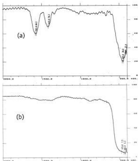
**Figure 1:** FT-IR spectra of (a) as synthesized zinc acetate film (b) ZnO NPs thin-film annealed at 400 °C.
