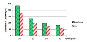
Fig.13.d. execution time for ILS method compared with line scan method where r=33cm  $\,$
