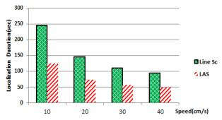
Fig.14.c. Execution time for LAS method compared with line scan method where r=23cm
