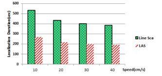
Figure 14.a. Execution time for LAS method compared with line scan method where r=3cm
