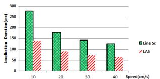
Fig.14.b. Execution time for LAS method compared with line scan method where r=13cm
