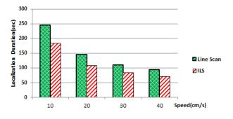
Fig.13.c. Execution time for ILS method compared with line scan method where r=23cm  $\,$
