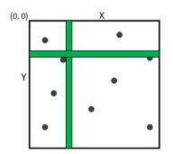
Fig.2.The line scan method, tow spotlights do scan horizontally and vertically
