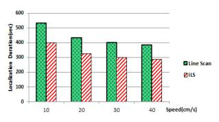
Fig.13.a. execution time for ILS method compared with line scan method where r=3cm  $\,$
