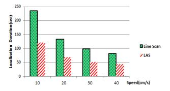
Fig.14.d. Execution time for LAS method compared with line scan method where r=33cm
