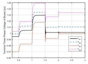
Fig. 10. Terminal three-phase voltage of buses
