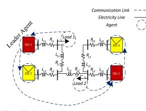
Fig. 6. Simulated microgrid structure
