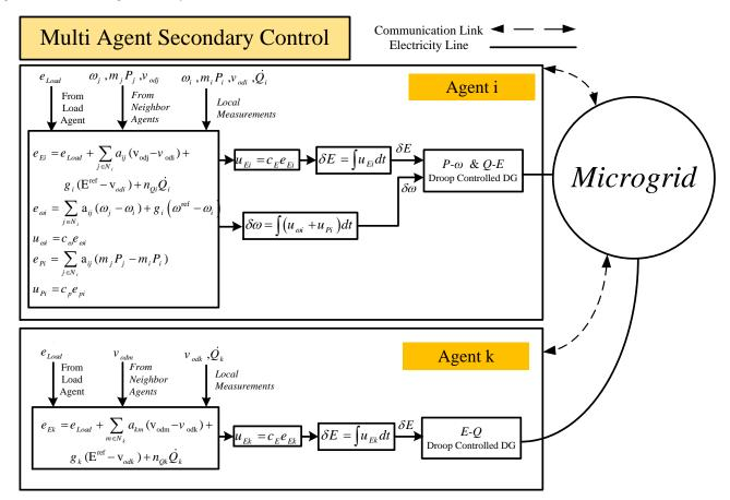
Fig. 5. Multi-agent based microgrid secondary control in islandedmode
