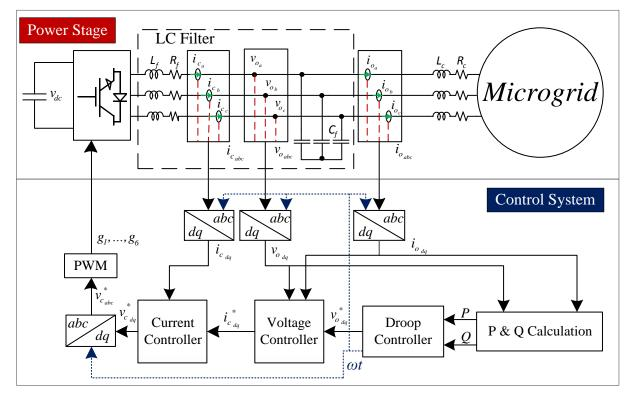
Fig. 1. Power stage and control system of the dispatchable units[8]
