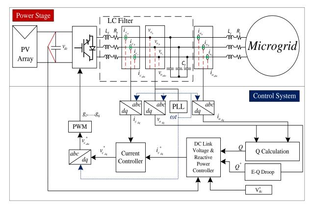
Fig. 2. Power stage and control system of the PV systems[8]
