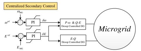
Fig. 4. Centralized microgrid secondary control in islandedmode[8]
