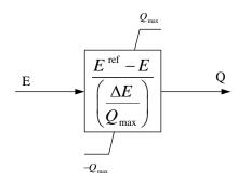
Fig. 3. E - Q droop blockdiagram[8]
