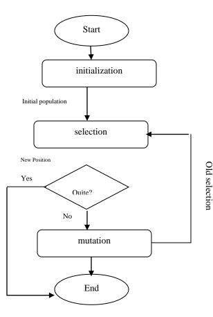
Figure2- Process flowchart genetic algorithm
