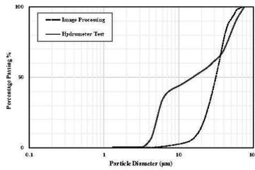
Fig. 7 Comparison of fine soil gradation curve obtained from hydrometer and static image processing methods
