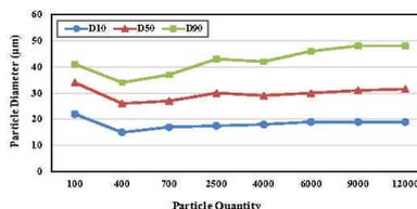
Fig. 10 The Effect of the number of sample particles on result accuracy
