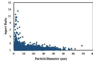
Fig. 8 Correlation between size of particles and aspect ratio
