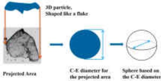
**Figure 5:** The definition of a sphere equivalent to a three-dimensional particle [5]
