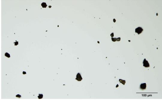
**Figure 1:** Microscopic image of fine soil particles
