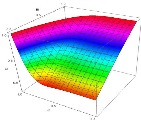
**Figure 7:** Heat transfer rate with respect to fin base temperature and Biot number with  $N_r = 1$  for any value of  $\alpha$ .
