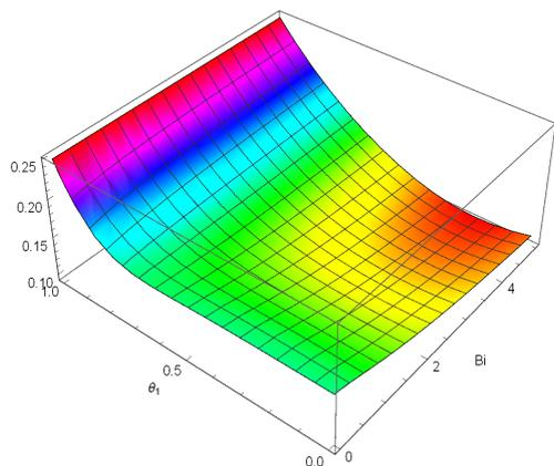
**Figure 9:** Fin efficiency with respect to fin base temperature and Biot number with  $N_r = \alpha = 1$ .
