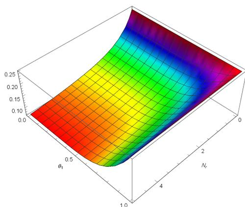
**Figure 10:** Fin efficiency with respect to fin base temperature and radiation-conduction number with  $Bi = \alpha = 1$ .
