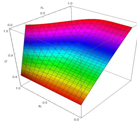
**Figure 8:** Heat transfer rate with respect to fin base temperature and radiation-conduction number with  $Bi = 1$  for any value of  $\alpha$ .
