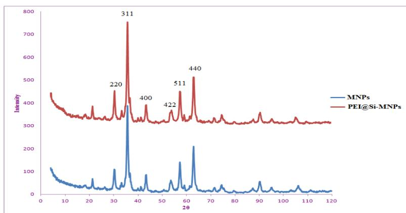
**Fig. 2.** XRD patterns of  $\text{Fe}_3\text{O}_4$  MNPs and PEI@ Si-MNPs
