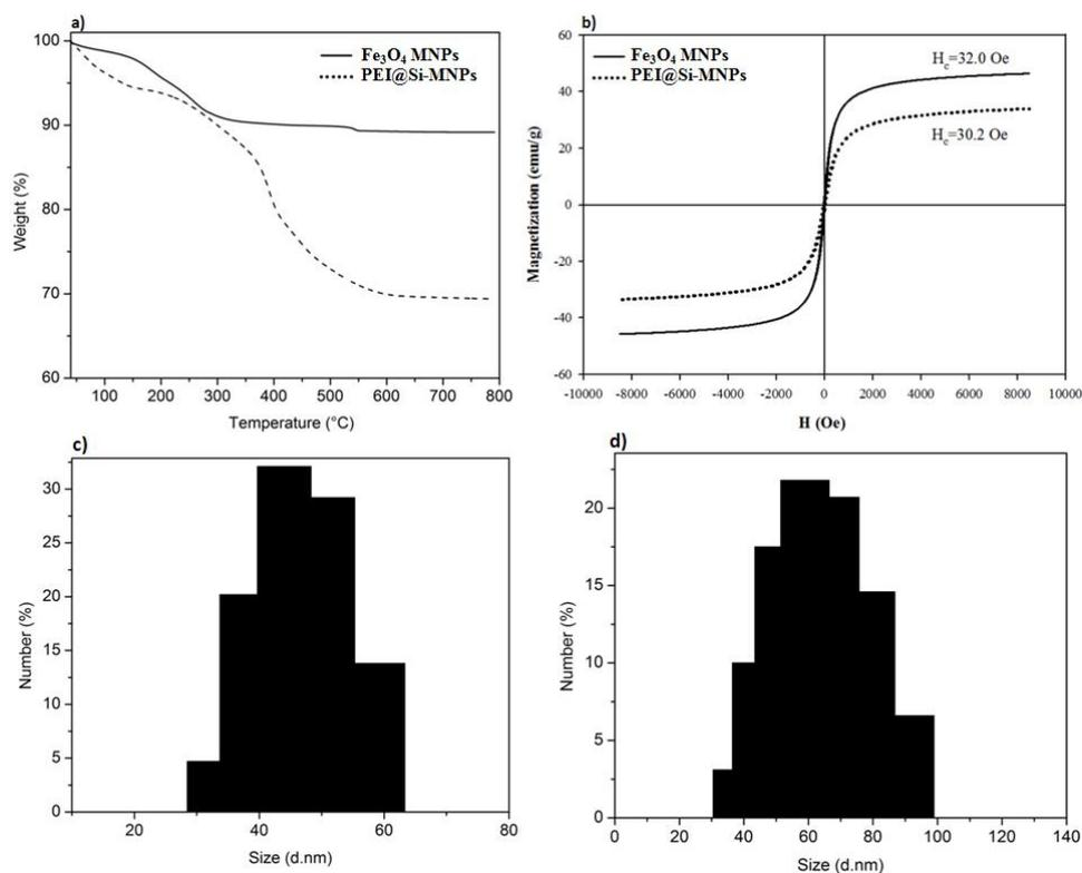
**Fig. 4.** a) TGA of Fe<sub>3</sub>O<sub>4</sub> MNPs and PEI@Si-MNPs, b) Hysteresis loops of MNPs and PEI@ Si-MNPs, c) HDs sizes of Fe<sub>3</sub>O<sub>4</sub> MNPs and d) PEI@Si-MNPs
