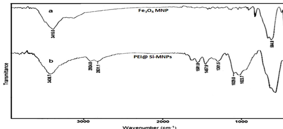
**Fig.1.** FT-IR spectrum of  $\text{Fe}_3\text{O}_4$  MNPs and PEI@Si-MNPs
