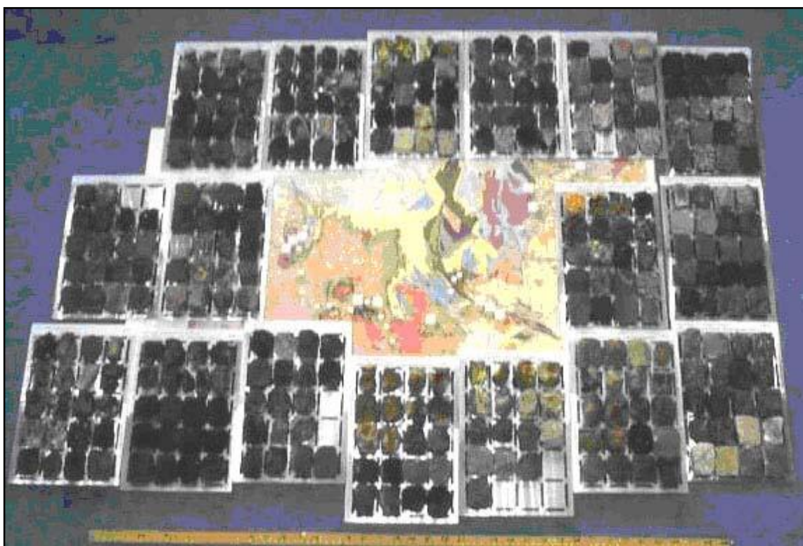
Figure 12. Lithotheque representation of deposits and lithology in the important Alligator Rivers uranium province in northern Australia.
