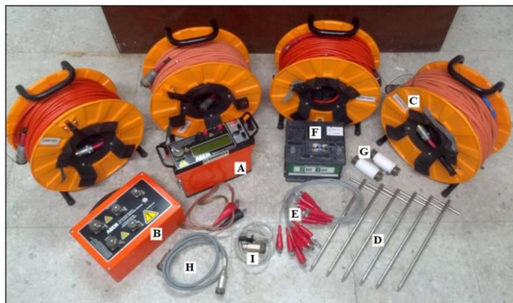
Fig 8. ERT equipment set-up: A. Main instrument of Terrameter (SAS 4000); B. Electrode selector model (ES10-64C); C. Electrode Cable rolls; D. Steel electrodes for data acquisition; E. Connectors cable-electrode; F. Battery for current supply; G. Cable connectors; H. Terrameter and electrode selector connector and I. Data transferring cable from Terrameter to laptop.
