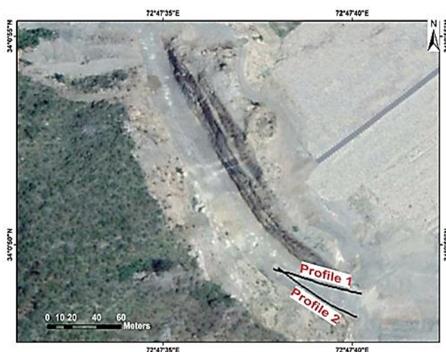
Fig 9. Plan showing location of imaging-based ERT profiles (1 and 2)
