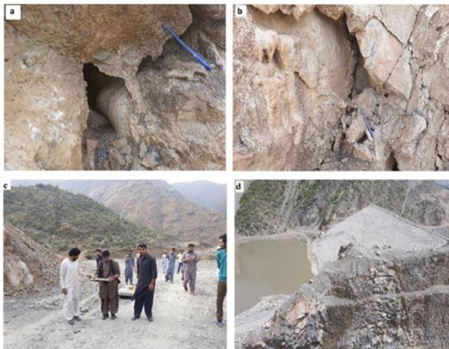
Fig 2. Karstic features observed on the surface near dam site. (a) Cavity formed due to dissolution of limestone (b) Limestone dissolution developing cavities and cracks (c) GPR data acquisition in the study area and (d) Gadwalian Dam main reservoir view
