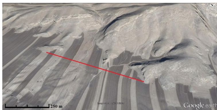
Fig 5. Google earth image of proposed section suitable for the construction of an underground dam on the agricultural area with a length of 800 m and a wall height of 30 m, site 3 of Figure 4.
