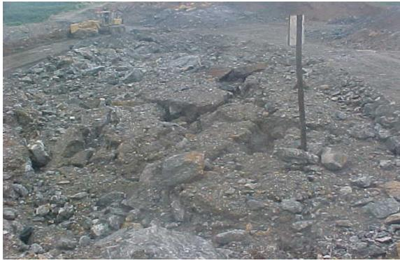
Fig 5. Muckpile heap along the back rows
