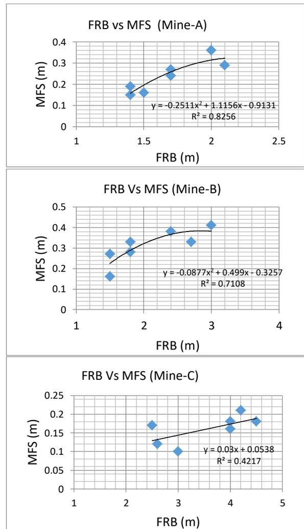
Fig 16. Front row burden (FRB) Vs Mean Fragment size (MFS) curve for Mine-A, B and C
