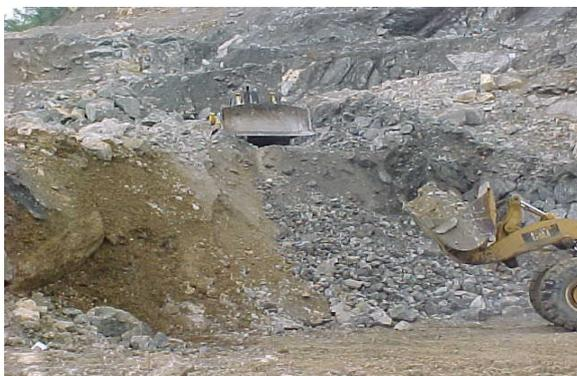
Fig 3. Front end loader assisted by dozer
