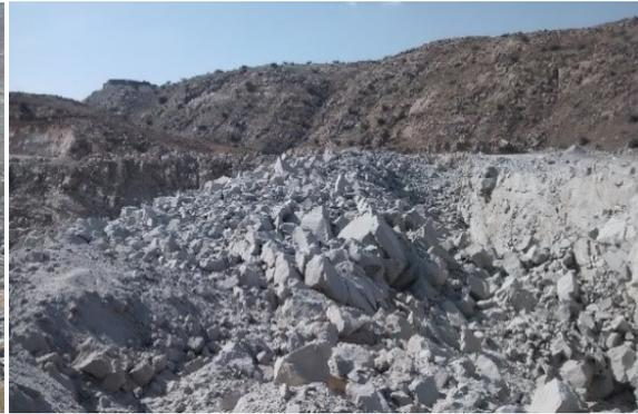
Fig 6. Back break at the final wall
