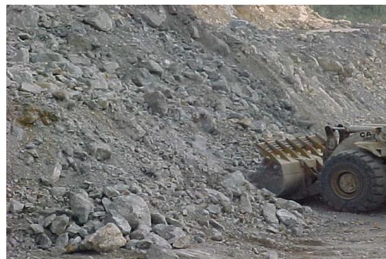
Fig 8. Blasted muck loading by FEL
