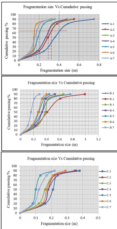
Fig 15. Composite fragment size distribution curve for Mine-A, B and C
