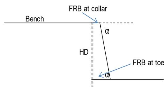
Fig 2. Shows differential FRB at top and bottom of bench ( $HD = FRB \tan(\alpha)$ ;  $FRB \text{ at bench toe} = FRB \text{ at crest} + (HD / \tan(\alpha))$ ;  $HD = \text{hole depth}$ ,  $\alpha = \text{bench slope angle}$ )
