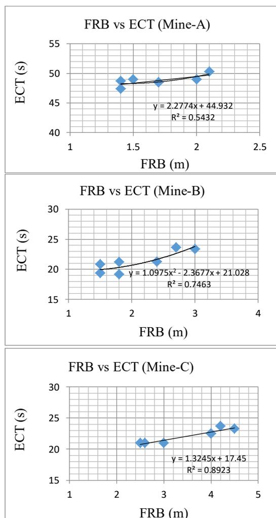
Fig 17. Front row burden Vs Excavator cycle time curve for Mine-A, B and C
