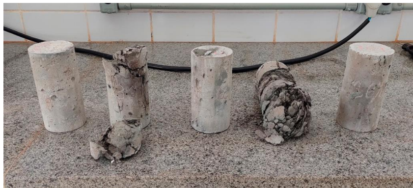
Fig. 2. The spalling during heating. Source: [26].
