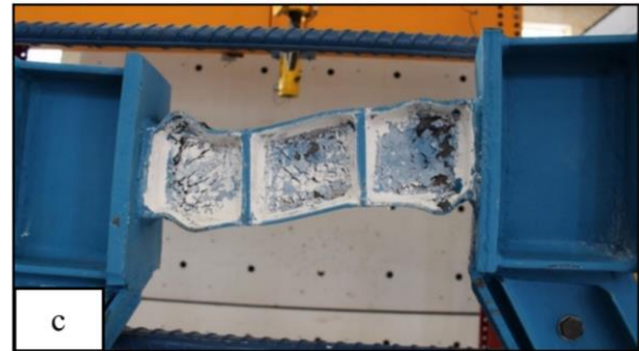
Fig. 15. Verification by experimental tests. (a) Before Test, (b) After Test, (c) Close ups fuse after test
