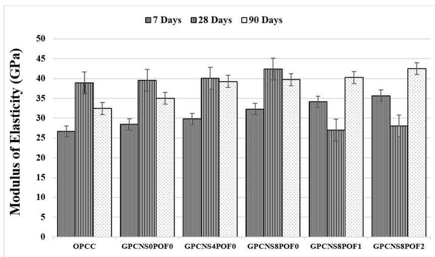
Fig. 2. The Modulus of Elasticity of the Specimens
