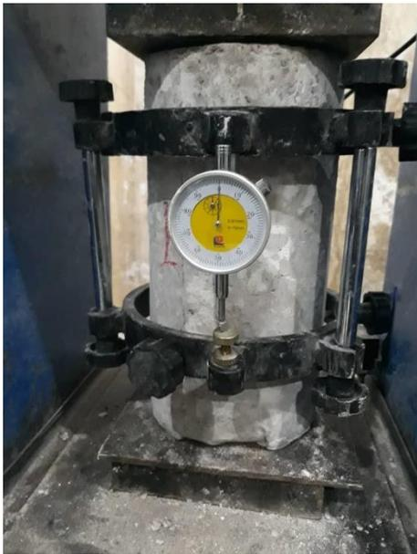
Fig. 3. Concrete Specimen Undergoing Modulus of Elasticity Test
