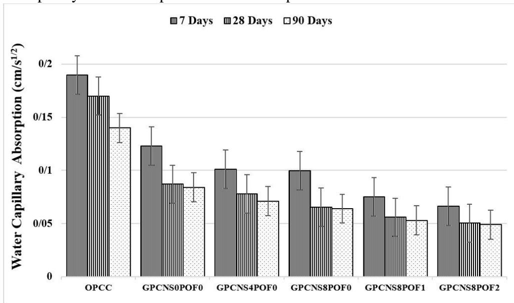
Fig. 5. The Water Capillary Absorption of the Specimens
