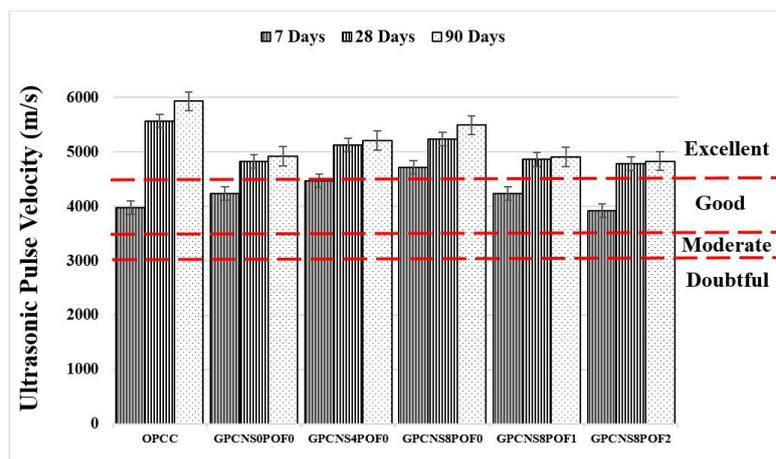
Fig. 4. The UPV of the Specimen
