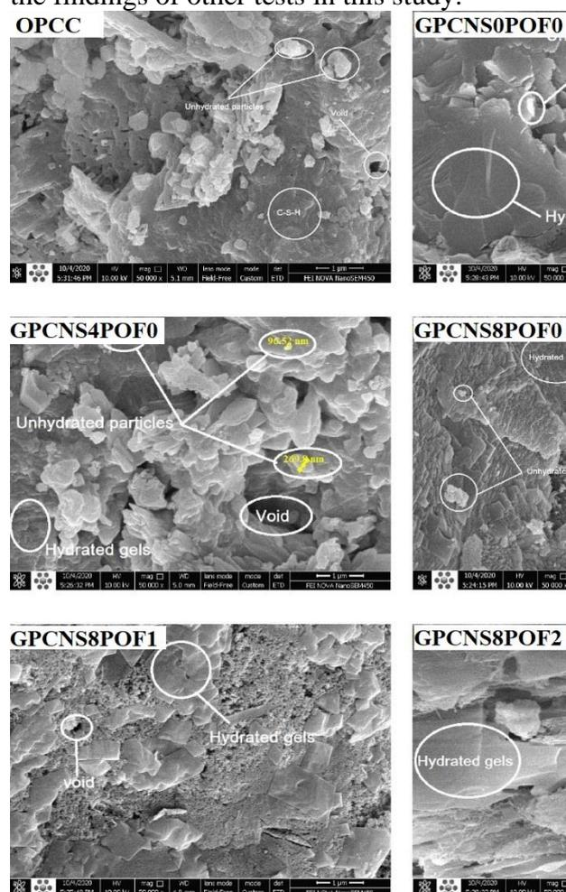
Fig. 6. SEM Image Under Room Temperature
