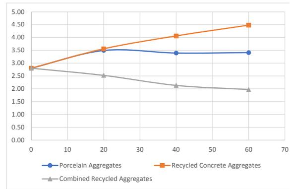
Fig. 21 water absorption changes according to replacement percentages
