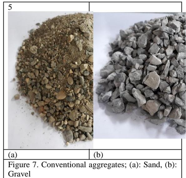
Figure 7. Conventional aggregates; (a): Sand, (b): Gravel
