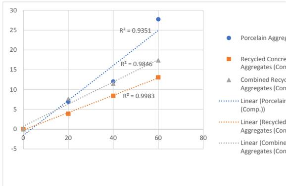
Fig. 10: Increase in compressive strength (%) trend lines
