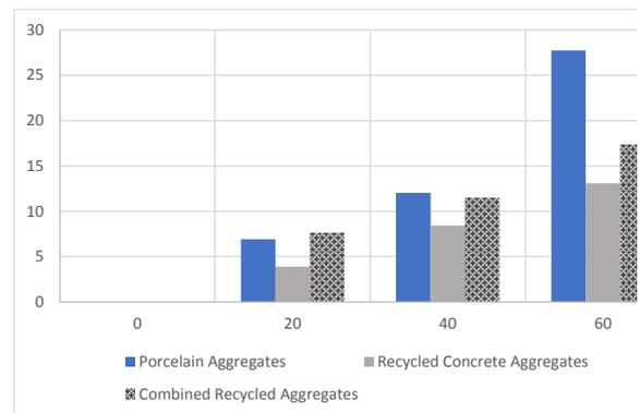
Fig. 9: Increase of compressive strength compared to the control sample (%), depending on the type of recycled aggregate and the percentage of replacement
