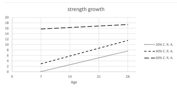
Fig. 14: Strength growth of concrete containing combined recycled aggregates
