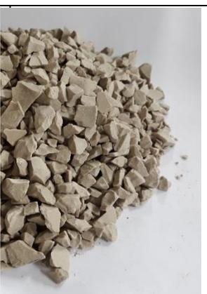
Figure 6. Recycled porcelain ceramic aggregates
