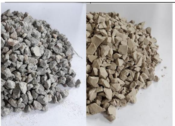
Figure 5. Recycled concrete aggregates
