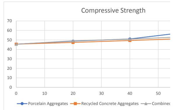
Fig. 8: Compressive strength changes of samples in terms of the aggregate replacement percentage
