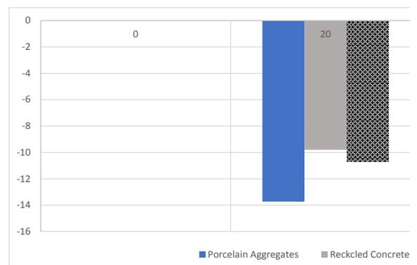
Fig .16 change of flexural strength in different percentage of aggregates replacement
