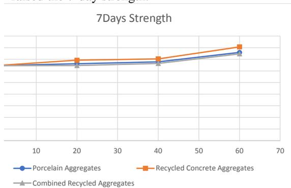
Fig. 11: 7-Day compressive strength changes of samples in terms of the aggregate replacement percentage
