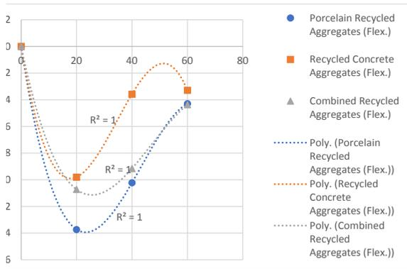
Fig. 17 Fitted curve on changes in flexural strength to replacement percentage
