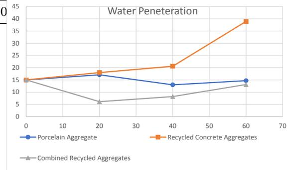
Fig. 19 water penetration changes according to replacement percentages
