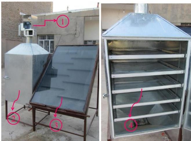
**Fig. 1.** The actual view of solar drying system: (1) centrifugal fan, (2) drying chamber, (3) solar collector, and (4) trays.
