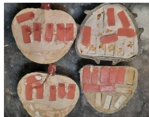
Figure 1. Muffled acrylic blocks. The right side is the flexible acrylic blocks and the left side is the heat-cure blockes
