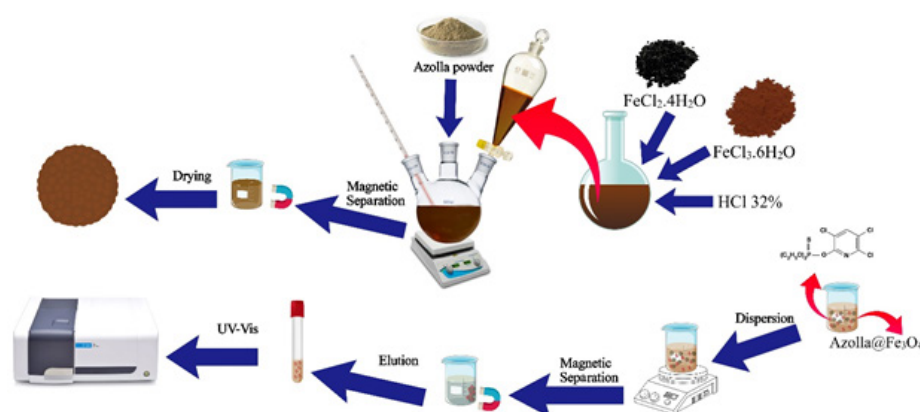
Fig. 3. Schematic for the application of azolla@Fe 3 O 4 NCs for the preconcentration of trace amounts of chlorpyrifos using MSPE prior to UV-Vis spectroscopy.
