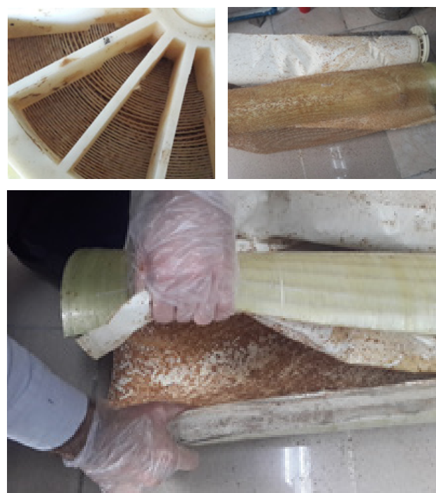
Figure 2. (clockwise) Example of the biofilm formed on the membranes from different angles.
