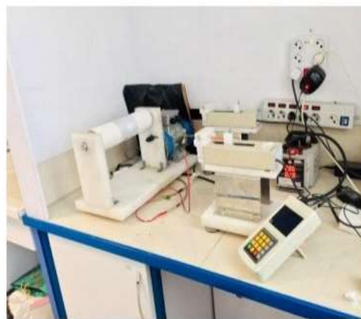
Figure 2: The electrospinning device used
