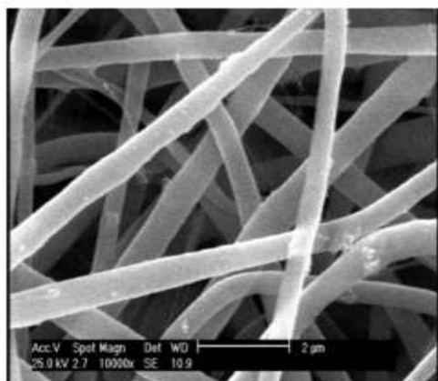
Figure 8: Scanning electron microscopy image for nano-fibrous membranes with 15% toluene by weight
