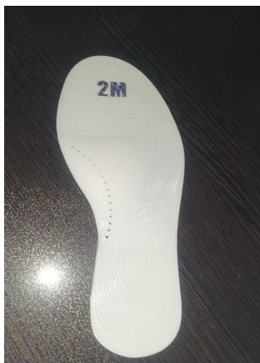
Fig.8.The final sample of the insole printed with flexi material, before being installed on the medical surface.
