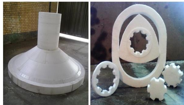
Fig. 10 View of two foam patterns made from two different castings.
