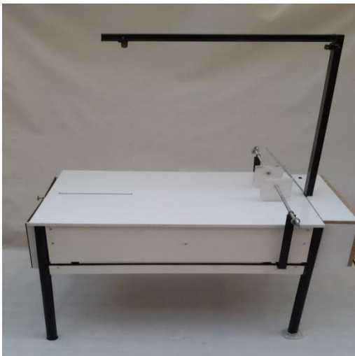
Fig. 9 Final assembly of semi-automatic foam cutting hot wire machine.
