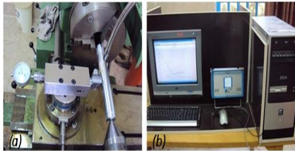
Fig. 3 Analog-to-digital dynamometer converter and display screen, with the workpiece secured in the device for the burnishing process.
