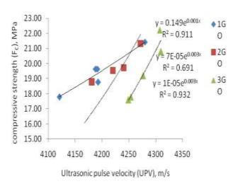
Fig. 5 Relationship between UPV and fc for Ogun riverbed sand (Day 7).
