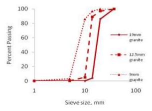
**Fig. 1** Coarse aggregate particle size distribution.
