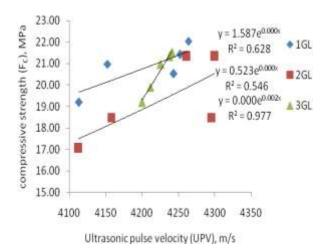
**Fig. 4** Relationship between UPV and f<sub>c</sub> for local drainage sand (Day 7).
