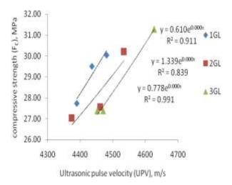
Fig. 6 Relationship between UPV and f<sub>c</sub> for local drainage sand (Day 28).
