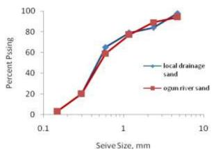
Fig. 2 Fine aggregate particle size distribution.
