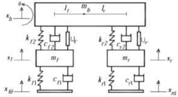
Fig. 1 Vertical model with active suspension.
