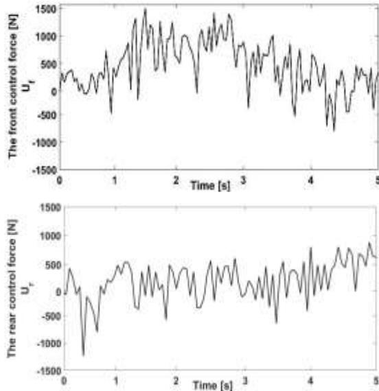
**Fig. 5** The front and rear actuators of active suspension. Power consumption of active suspension is determined as the following [18]:
