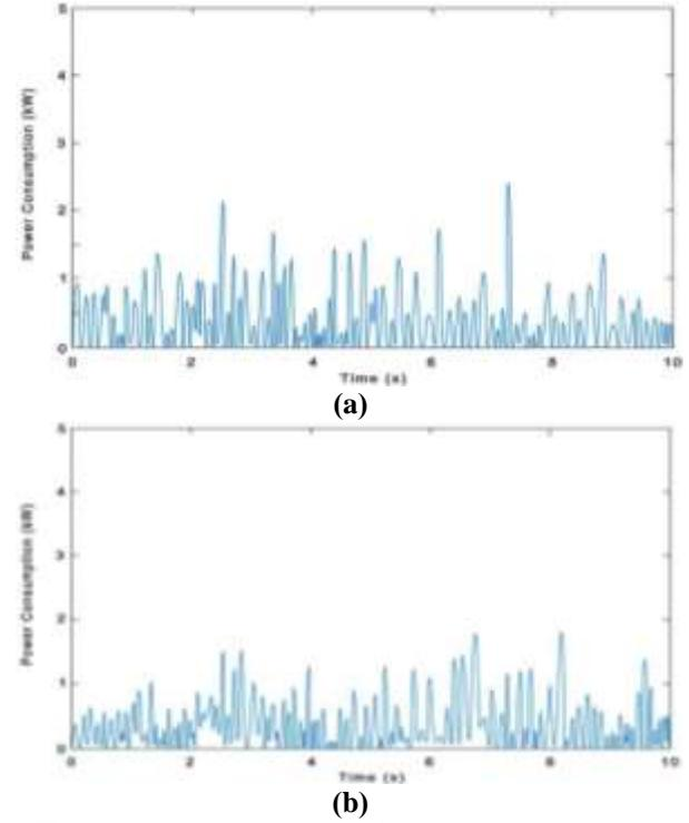
**Fig. 5** Power consumption of the controller system: (a): front suspension, and (b): rear suspension.
