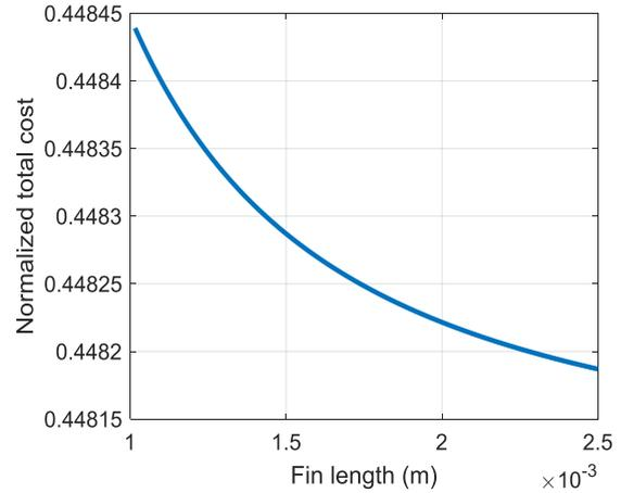
**Fig. 1** Effects of the fin length (c) on the thermal efficiency ( $\epsilon$ ) and normalized total cost ( $C_{total}^N$ ).
