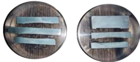
**Fig. 4** Specimens in mount for macrography
