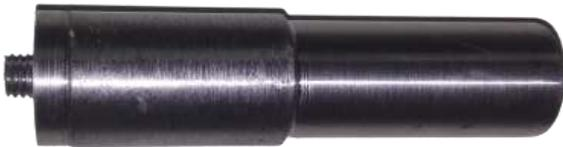
**Fig. 2** Photographs of FSP/FSW shoulder.
