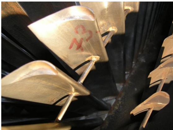
Fig. 9 Damping wire in blades.
