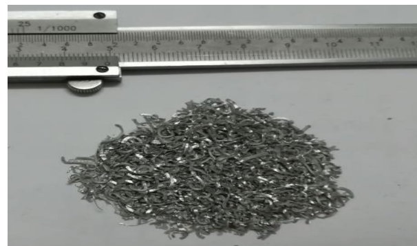
Fig. 1 Aluminum chips used in the friction stir extrusion process.
