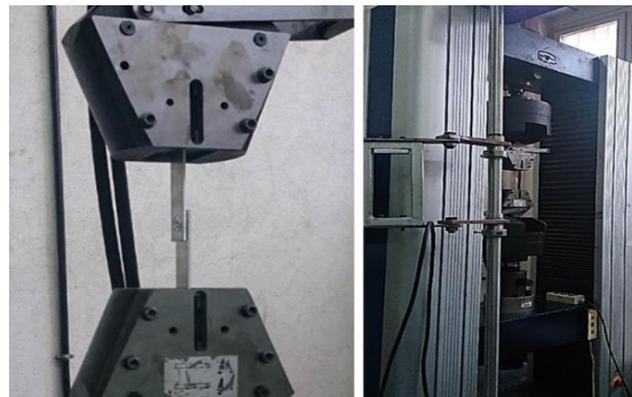
Fig. 5 Tensile test and sample placement at the machine.
