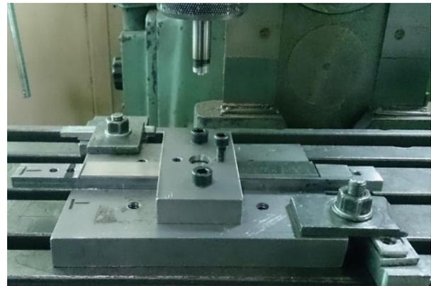
Fig. 4 The FSSW fixture on the milling machine table.
