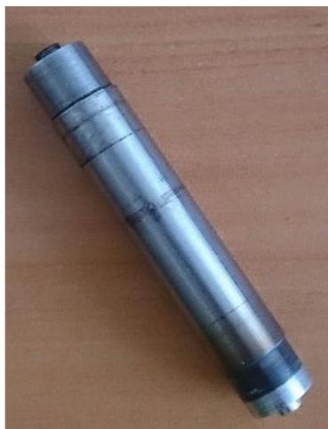
Fig. 3 FSSW tool used in the study.
