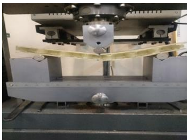
Fig. 2 The three-point bending fixture and its different components.
