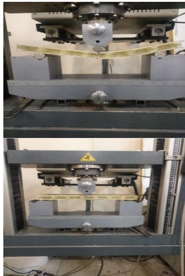
Fig. 10 The second specimen under the three-point bending load.
