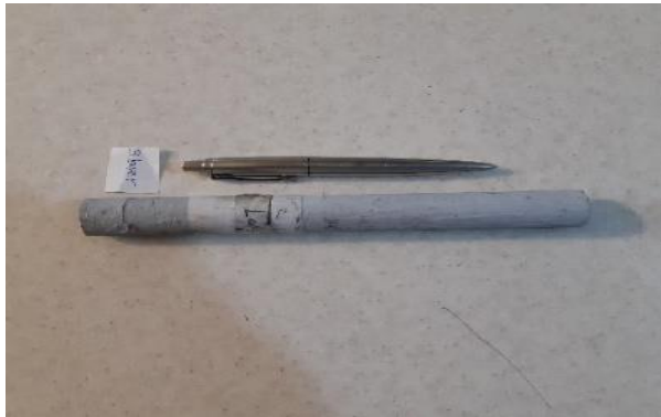
Fig. 4 The experimental specimen coated with mixed SiC/TiO 2 /SiO 2 particles.
