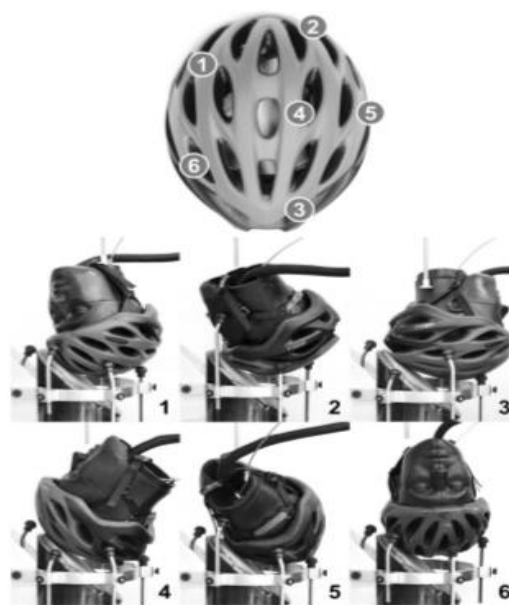
Fig. 2 Selected point for impact test [14].
