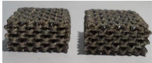
Fig. 12 Simple lattice structure after compressive test.
