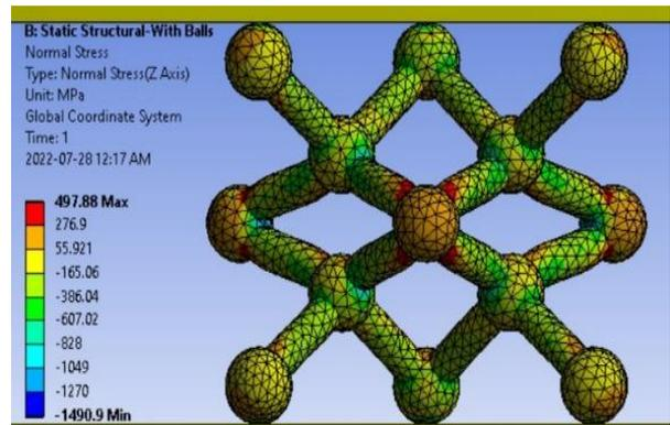
Fig. 9 Normal Stress in reinforced lattice structure.
