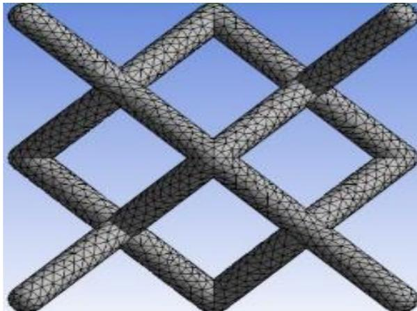
Fig. 6 4 Nodes rigid 3D shell mesh.
