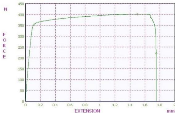
**Fig. 3** Force-displacement diagram of stainless steel 316L material.
