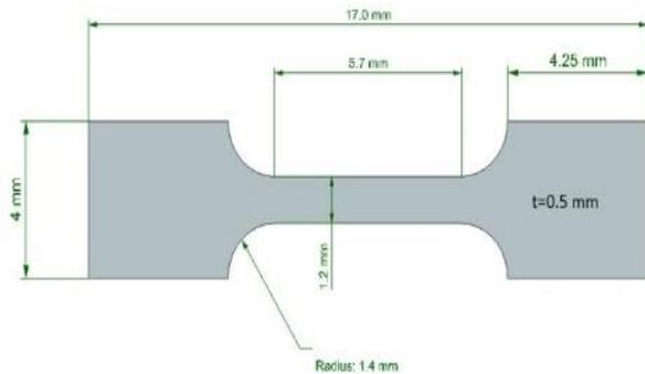
**Fig. 1** ASTM E8 – Sheet type tensile test specimen [12-13].
