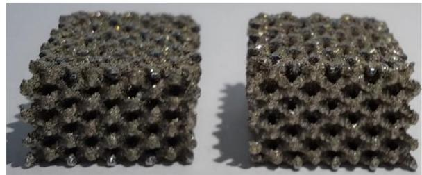
Fig. 13 Reinforced lattice structure after compressive test.
