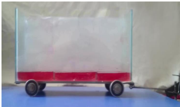
Fig. 1 The experimental mechanism considered for investigating the effect of baffles on the shallow water sloshing phenomenon.
