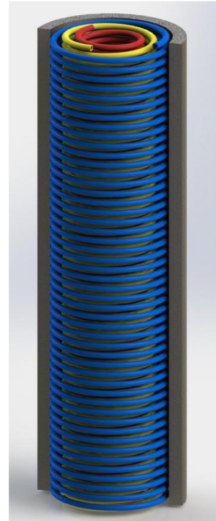
Fig. 5 Scheme of the helical steam generator.
