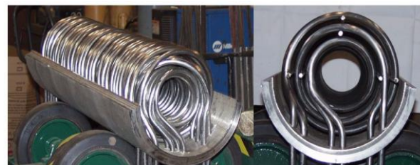
Fig. 4 Photographs of SG coil bundle arrangement [10].
