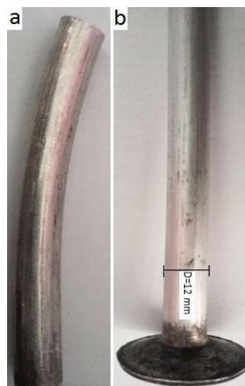
Fig. 5 Bent and defected sample (a), Perfect sample (b)
