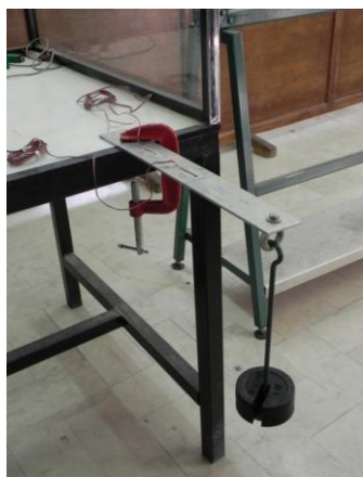
Fig. 5 Test setup of the aluminum strip, installed strain gauges, and loading of the strip plate
