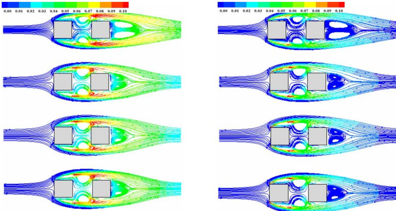
**Fig. 4** The time-averaged streamline colored by turbulence kinetic energy (left side graphs) and turbulence kinetic energy dissipation (right side graph) for Reynolds number  $Re=2700, 16000, 40000, 70000$  from top to down, respectively and the distance between the cylinders,  $G=1$
