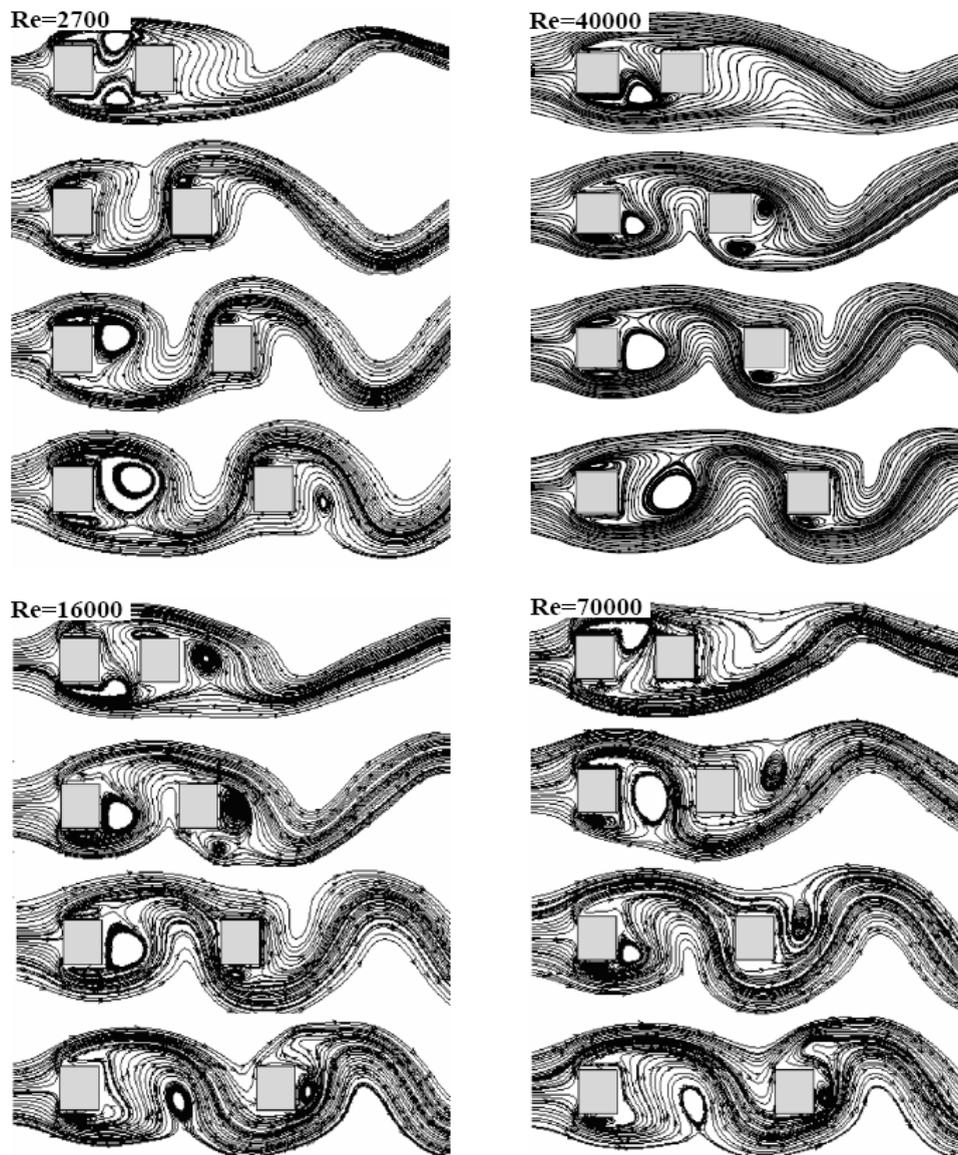
Fig. 3 Instantaneous streamlines vicinity of cylinders for different Reynolds numbers and the distances between the cylinders
