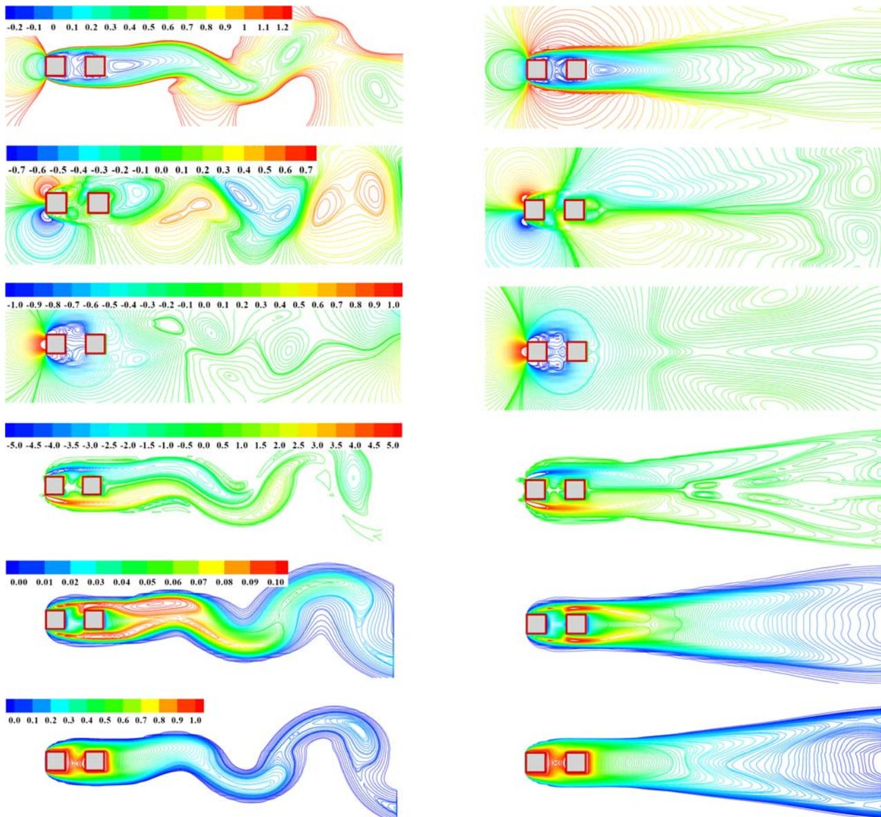
**Fig. 2** Instantaneous (left side graphs) and time-averaged (right side graphs) contours from top to down; X-velocity component; Y-velocity component; pressure; Z-vorticity component; turbulent kinetic energy and temperature, respectively around the cylinders for Reynolds number,  $Re=2700$  and distance between the cylinders,  $G=1$
