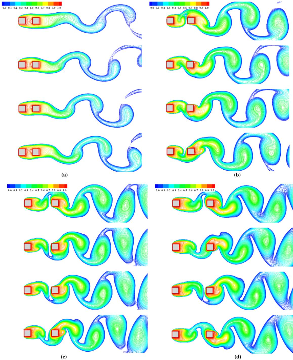
**Fig. 9** Instantaneous isotherm pattern contours vicinity of cylinders for the Reynolds number  $Re=2700, 16000, 40000, 70000$  from top to down, respectively: (a)  $G=1$ ; (b)  $G=2$ ; (c)  $G=3$ ; (d)  $G=4$
