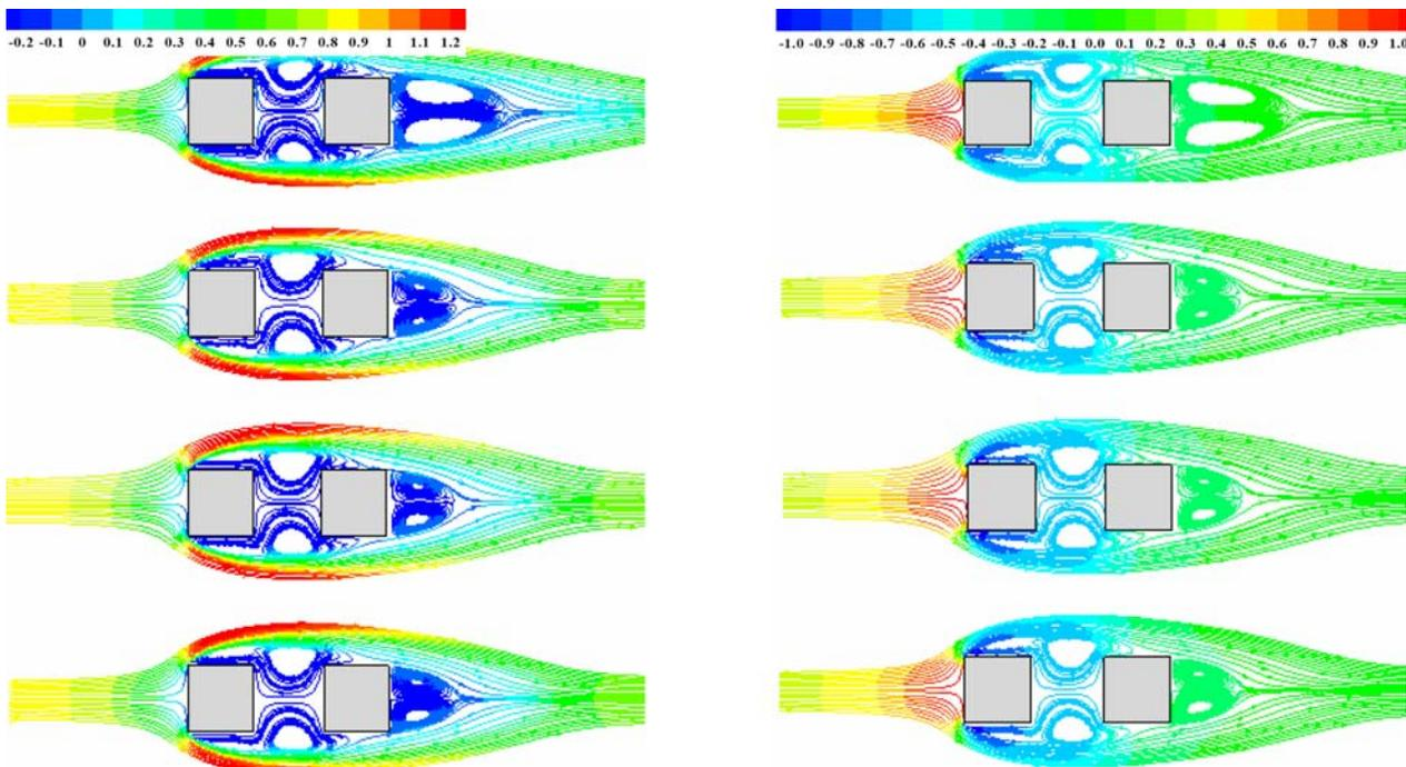
**Fig. 5** The time-averaged streamline colored by X-velocity component (left side graphs) and pressure (right side graph) for Reynolds number,  $Re=2700, 16000, 40000, 70000$  from top to down, respectively and the distance between the cylinders,  $G=1$
