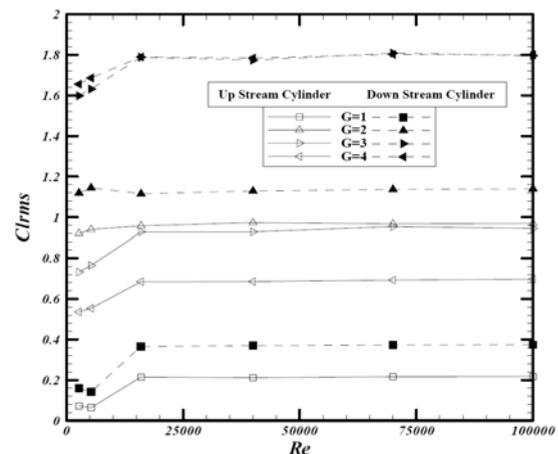
Fig. 6 Variation of RMS of lift force versus Reynolds number
