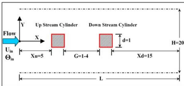
Fig. 1 Computational domain for flow around the square cylinders
