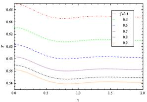
**Fig. 11** Transient response of the viscoelastic damper. The transient force on the plates is shown for We = 1, Re = 0.1,  $\zeta \in [0.4,0.9]$  and  $\varepsilon = 0.04$
