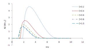
**Fig. 5** Stable steady-state solution branches  $N_2^s(We, \zeta)$  as function of We for  $\zeta \in [0,1]$  and  $\varepsilon = 0.04$ . Note that the branches are symmetric with respect to the horizontal axis
