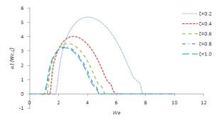
**Fig. 8** Stable steady-state solution branches  $u_1^S(We, \zeta)$  as function of We for  $\zeta \in [0,1]$  and  $\varepsilon = 0.04$ . Note that the branches are symmetric with respect to the horizontal axis
