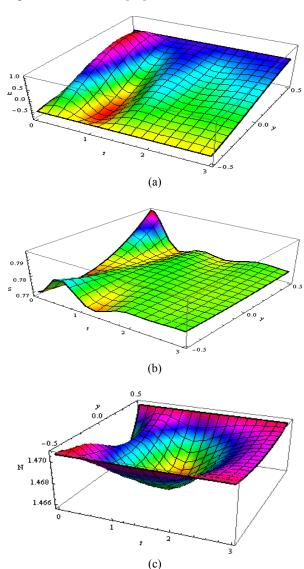
**Fig. 10** Transient behavior of flow in the precritical range  $(We < We_{c1})$ . Evolution of solution towards the base flow for Re = 0.1, We = 1,  $\varepsilon = 0.04$  and  $\zeta = 0.2$ . In this case, since  $Re > Re_0 = 0.0065$ , the behavior is oscillatory. Evolution of velocity (a), shear stress (b) and normal stress difference (c) are shown
