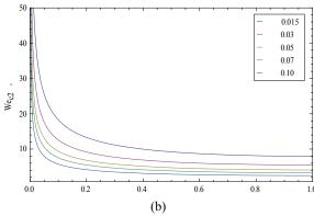
Fig. 3 Marginal stability curves for  $\epsilon \in [0.015,0.10]$  for the second critical weisenberg number  $We_{C2}$ . The curves are plotted against  $\zeta$  for the range [0,1]. Note that curves are symmetric with respect to  $\zeta = 1$ . The approximate curves based on the six-dimensional model system (B1) are shown in (a), and the exact curves are shown in (b)
