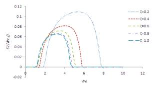
**Fig. 7** Stable steady-state solution branches  $S_2^S(We, \zeta)$  as function of We for  $\zeta \in [0,1]$  and  $\varepsilon = 0.04$
