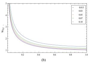
Fig. 2 Marginal stability curves for  $\epsilon \in [0.015,0.10]$  for the first critical weisenberg number  $We_{C1}$ . The curves are plotted against  $\zeta$  for the range [0,1]. Note that the curves are symmetric with respect to  $\zeta = 1$ . The approximate curves based on the six-dimensional model system (B1) are shown in (a), and the exact curves are shown in (b)
