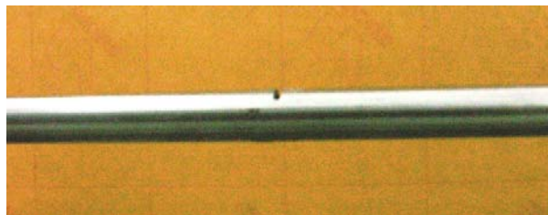
Fig. 9 Transverse crack like fault made on the shaft
