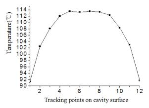
Fig. 3 Temperature distribution over the cavity surface of cavity plate
