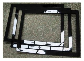
Fig. 8 TV Panel fabricated using variotherm injection technology
