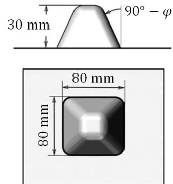
**Fig. 5** Dimensional characteristics of the formed sample
