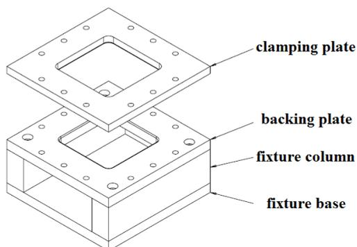
**Fig. 4** Components of the fixture in SPIF process
