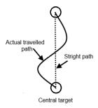
**Fig. 11** Direction Control. This is a measure to assess the person's ability to control COP toward the target. Direction Control Score is computed by dividing the intended straight path by the actual traversed path and multiplying the resultant in 100
