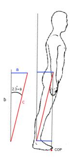
Fig. 9 Converting the angular limits of stability to a linear distance. The relation among the person's height, COP and limit of stability is shown by a triangle. The ankle is considered attached to ground as a part of that.
