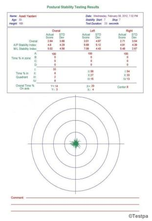
**Fig. 14** A sample of printed reports for postural stability protocol. The Stability Indices, standard Deviation for Mean Deflection, the time elapsed in each quadrant; zone, axis and origin are reported for overall conditions, left and right legs
